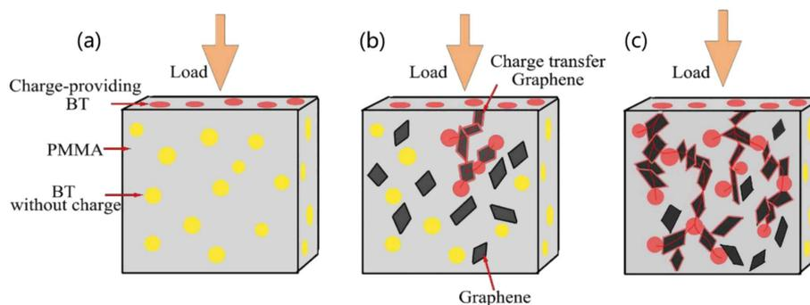
**Figure 12.** Improving mechanism of the piezoelectric coefficient of the G/BT/PMMA bio-piezoelectric composites by graphene addition: a) no graphene is added, b) a small amount of graphene is added and c) sufficient graphene is added [147]
