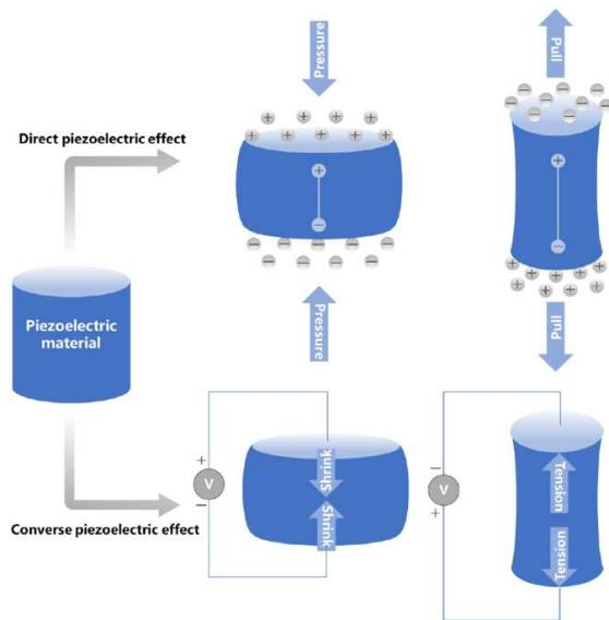
Figure 4. Power-to-electricity conversion of piezoelectric materials
