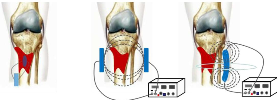
Figure 2. Implanted power stimulation (a), invasive tissue stimulation (DC/pulse generator + invasive electrode) (b) and non-invasive tissue stimulation (capacitive coupler + inductively coupled stimulation) (c)
