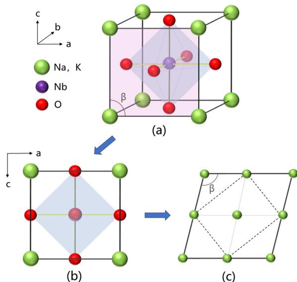
**Figure 9.** The unit cell structure of KNN
