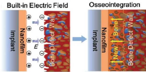
**Figure 6. Illustration of rapid osseointegration between electropositive implant and electronegative bone interaction [48]**
