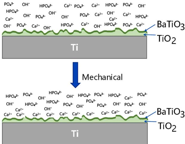
**Figure 8.** A periodic load is applied to generate a negative charge on the surface of BT, which can attract  $\text{Ca}^{2+}$  to gather on the coating surface
