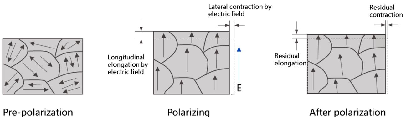
**Figure 7. Schematic diagram of polarization process of BT**
