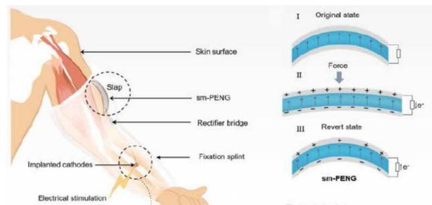
Figure 5. Schematic diagram of self-powered electrical stimulation for bone repair [47]
